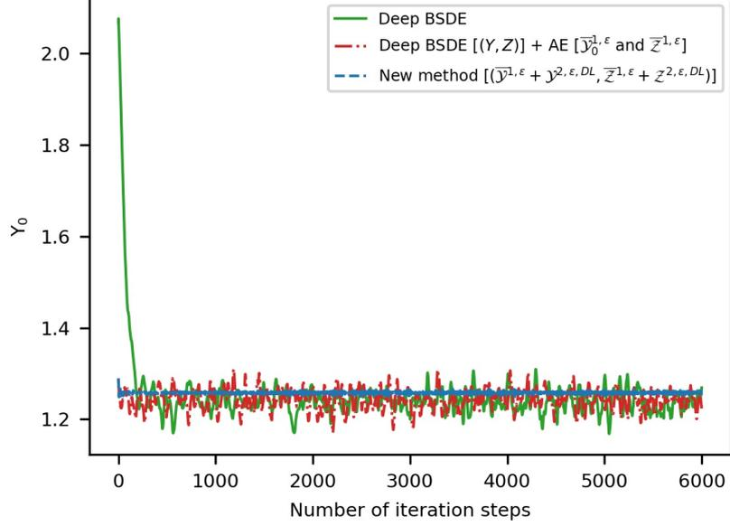
Figure 8: Approximate values of  $Y_0$  (true value: 1.26) and number of iteration steps (1-dim option pricing model with CVA, OTM case)
